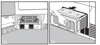
Do not be alarmed by the amount of fluff. It is not due to excessive wear caused by the dryer. All fabric looses fluff when drying but it goes un-noticed in the air. In a tumble dryer it simply collects in the filter. Clean it with a brush and rinse it under the shower if necessary.
